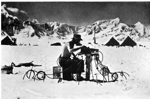
Fig. 3. Temperature measuring equipment installed at Austin Station on the upper Seward Glacier (see text, p. 479)
