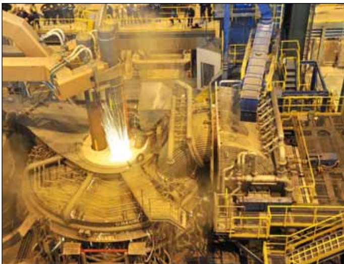
The hot testing was carried out on the arc steel-smelting furnace, ladle furnace unit, steel vacuum degassing unit, and continuous casting machines.
