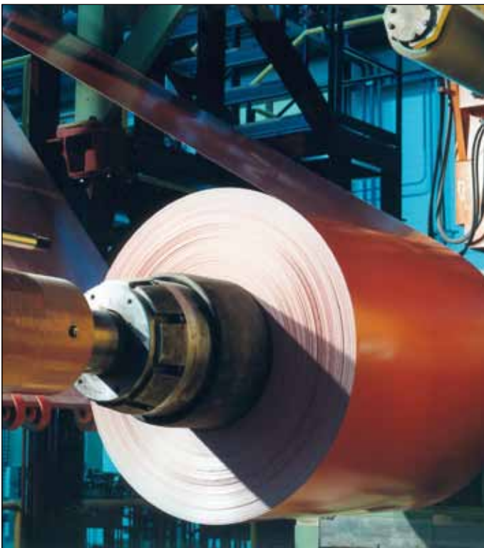
The paint- and film-coated steel is supplied in the form of coil, slit strip and cut-to-length sheets.
