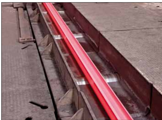
Section rolled on a rolling mill for medium-sized products from Siemens.
