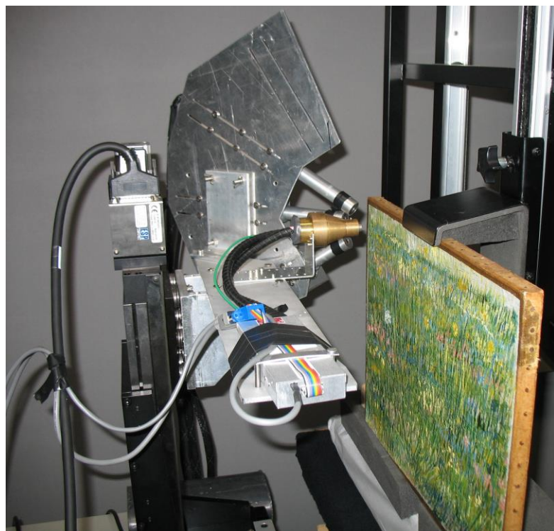
Figure 1. In-house build MA-XRF scanner of the University of Antwerp while investigating Vincent van Gogh's Patch of Grass.
