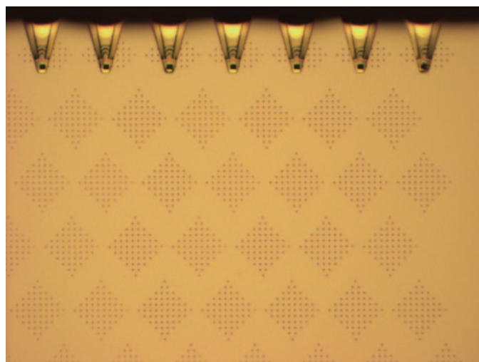
Figure 8: Light microscope image of arrays of dots in a diamond-shaped pattern created by the NLP 2000.
