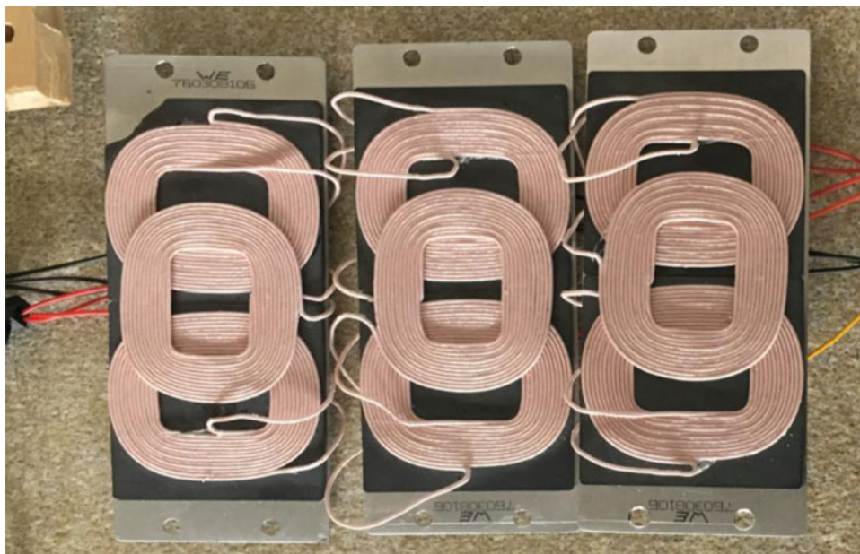
Fig. 15. The 3 × 3 coil array structure.
