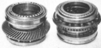
40 Weir W 6 rotor hub gears and ratchet free wheels to give correct phasing of rotors
