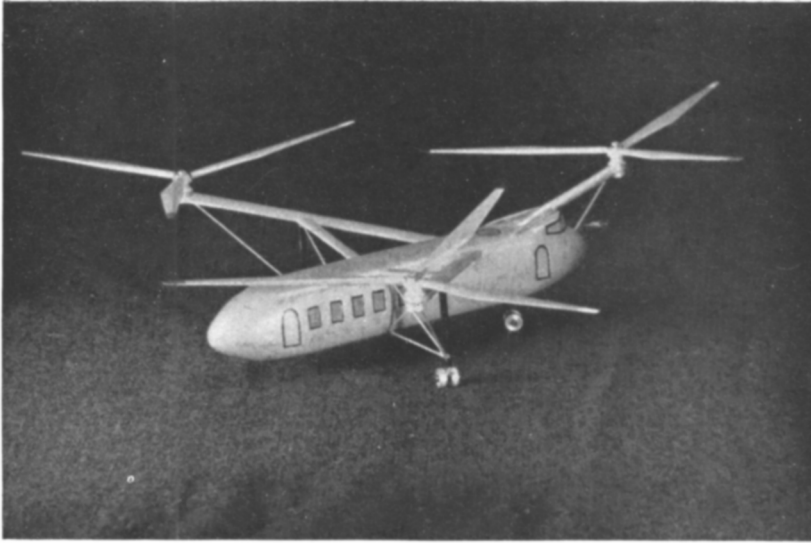
51 W 11 Air Horse model The full scale machine is now under construction With Rolls Royce Merlin engine this aircraft will have a payload of three tons
