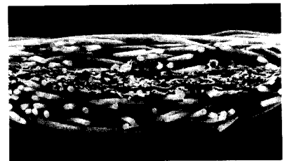
Cross-section of CONTROL Cover Gown Fabric
