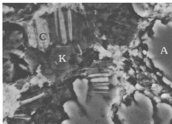
Figure 8. Back-scattered electron image of lamellar chlorite (C) pseudomorphous after blocky kaolinite (K). Well R37879, 4570 m. Field of view = 45 \mu\text{m} . A = albite.
