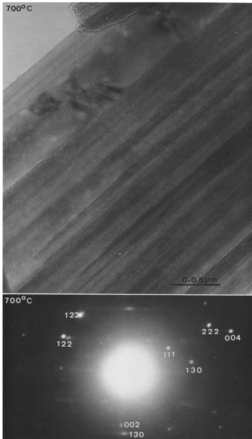
Figures 7 and 8. (7) Coalescence between fibrils has started at 700°C and in the coalesced areas, many voids, round and sometimes elongated, are included. (8) In the SAD pattern at 700°C the (00l) spots of chrysotile are almost absent, however, the 14–15 Å spots are visible together with other spots easily identified as being from forsterite.
