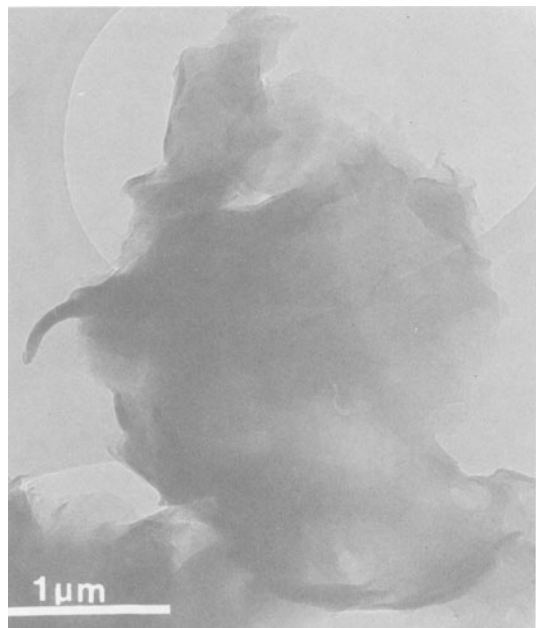
Figure 6. TEM image of a smectite flake in the clay fraction showing the typical "cornflake" texture.
