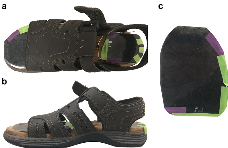
Figure 1. Sandal with nanocomposite sensors on the hindfoot and forefoot regions of the insole viewed from (a) above and (b) the medial side. (c) An individual nanocomposite sensor.
