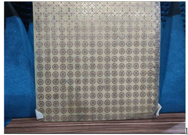
Figure 12. Fabricated prototype metamaterial absorber.
