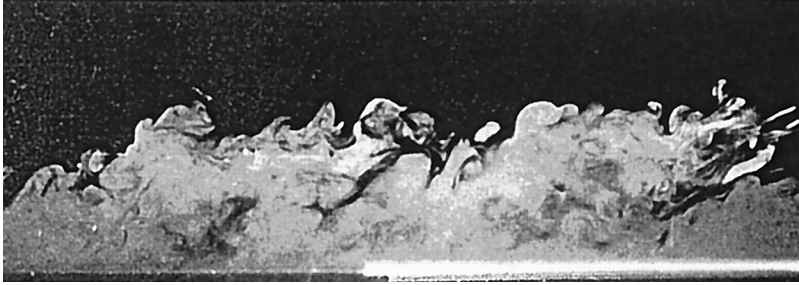
Figure 1. Material wall-bounded turbulent structures visualized with smoke. Reproduced from Falco (1977) with the permission of AIP Publishing.
