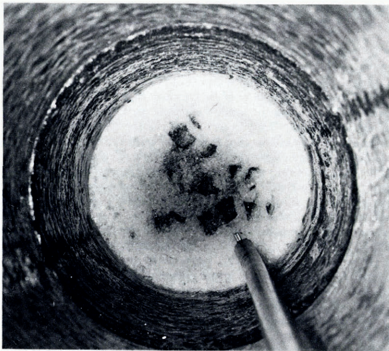
Fig. 6. Photograph taken of bedrock at the base of a 337 m hole drilled on the Agassiz Ice Cap, northern Ellesmere Island in May 1977. The bore-hole diameter is 16 cm.
