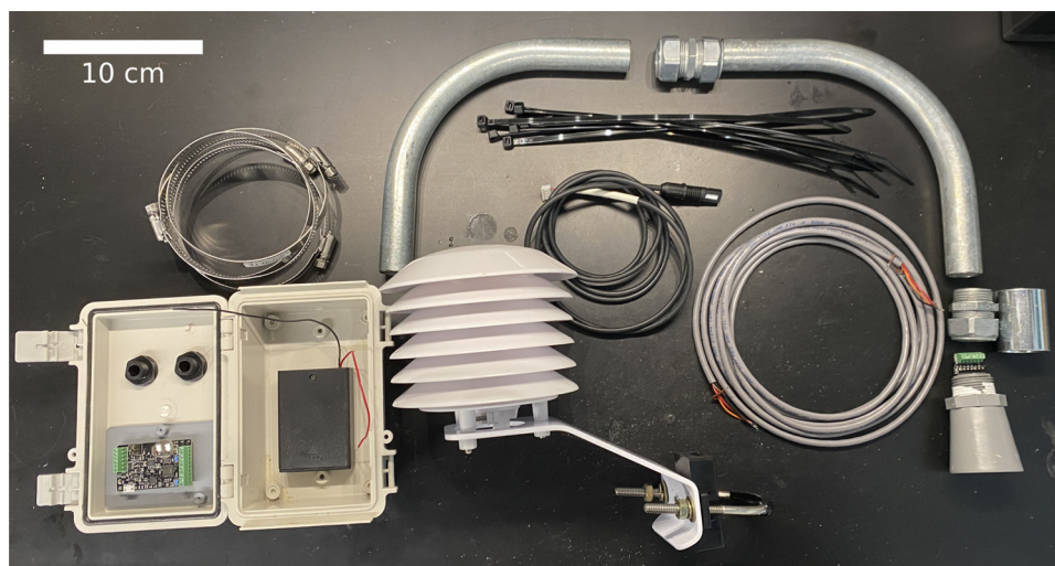
Figure 4. Materials to assemble the sensing component of the automated ablation stake. Lower left: Box with cable glands, Margay data logger and 3 × AA battery pack. Upper left: 4 × hose clamps. Upper right: Conduit inverted U with compression connector (top) and compression adapter (right); compression adapter threads onto the straight connector (far right) to attach to the MaxBotix ultrasonic rangefinder (lower right). Above middle: cable ties. Center (black cable): Temperature and relative-humidity sensor. Center right (gray cable): Cable to attach the MaxBotix ultrasonic rangefinder to the data logger. Lower middle: Solar radiation shield. Not pictured: MaxTemp temperature correction for the ultrasonic rangefinder; mounting hardware for the ultrasonic rangefinder.
