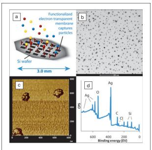
Figure 1. Dune Sciences' SMART grids products capture and immobilize materials for nanoscale characterization using a wide range of analytical tools: (a) SMART grids; (b) transmission electron micrograph of silver nanoparticles (AgNPs) captured on NanoPLUS™ grids; (c) atomic force micrograph of degraded AgNPs on NanoPLUS grid; and (d) x-ray photoelectron spectroscopy results of Ag NPs on
