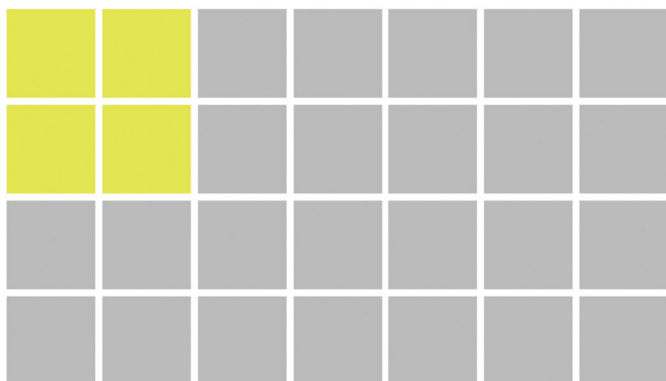
Figure 3: Example of binning. When the full lateral resolution of a sensor array (either CCD or CMOS) is not required, the charge from several sensors can be combined into a single value. This is called binning. The yellow sensors indicate a 2 \times 2 binning to create a “super” sensor. By combining the signal from 4 adjacent photosensors, the signal-to-noise ratio is increased.
