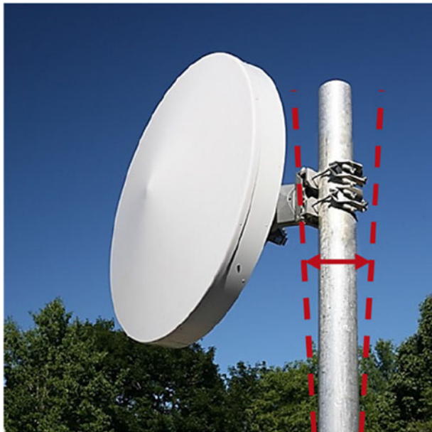
Figure 1. Cassegrain reflector antenna with small boom movements.
