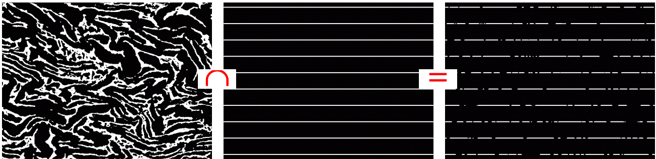
FIG 3. Intersection of a grid with the binary image of the microstructure to give the intercepts.
