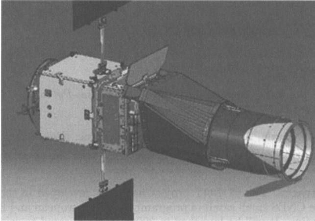
Figure 1. The design of the COROT satellite: the left part is the PROTEUS platform. The telescope is in the middle part, while the baffle, with its cover, is seen on the right side.
