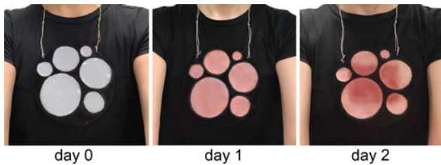
Figure 13. The interactive pendant changes color from light pink to dark pink as the bacterial dye responds to the rising temperature of the heater.
