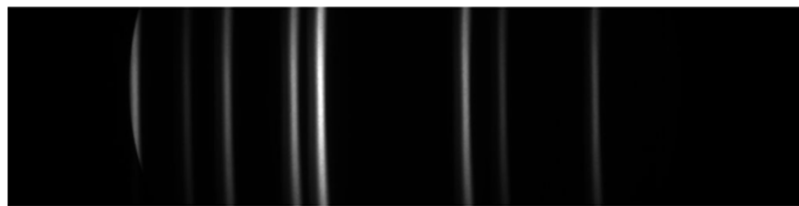
Figure 1. An example of detected spectral frame showing Ne-Ar emission lines in the 620–660 nm range.
