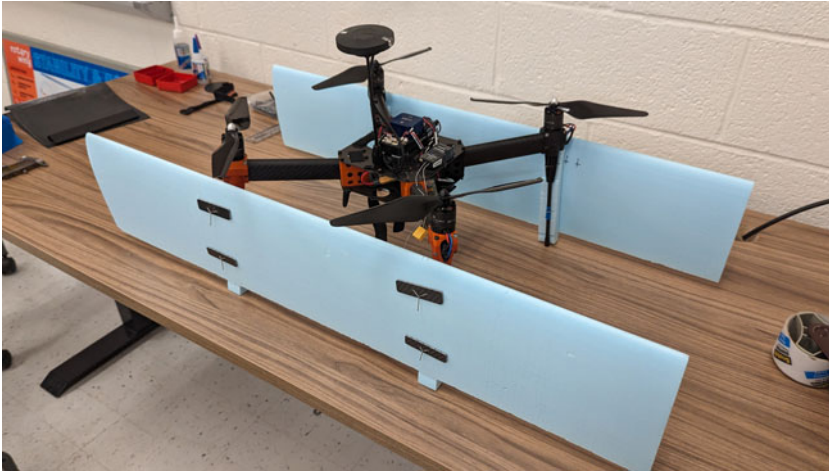
Figure 1. Quadrotor showing Hexsoon EDU-450 frame and custom foam wings.
