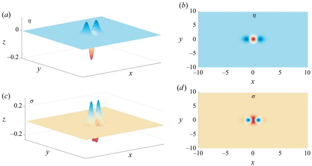
Figure 5. Steady weakly nonlinear wave-free solutions defined in (3.2). Panels (a–b) the nonlinear free surface,  $\eta(\mathbf{x})$  for  $a = 0.1$ ,  $Fr = 1.0$ . Panels (c–d) the forcing,  $\sigma(\mathbf{x})$ .
