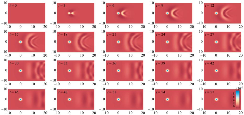
Figure 9. Fully nonlinear moving-pressure time-dependent solution for  $\eta_f(\mathbf{x}, t)$ ,  $x \in [-10, 30]$ ,  $y \in [-10, 10]$ , with  $\sigma_{press}(\mathbf{x})$  given in (4.7) for  $\eta_g(\mathbf{x})$  in (4.9),  $Fr = 1.0$ ,  $a = 0.01$ .
