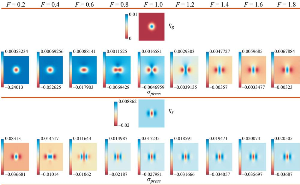
Figure 6. Fully nonlinear moving-pressure problem as  $Fr$  is varied. Each panel is plotted in the range  $x \in [-10, 10]$ ,  $y \in [-10, 10]$ . First and second rows: wave-free profile  $\eta_g(\mathbf{x})$  and corresponding  $\sigma_{press}(\mathbf{x})$ , respectively. Third and fourth rows: wave-free profile  $\eta_s(\mathbf{x})$  and corresponding  $\sigma_{press}(\mathbf{x})$ , respectively. In both cases  $a = 0.01$  (see (4.9)).
