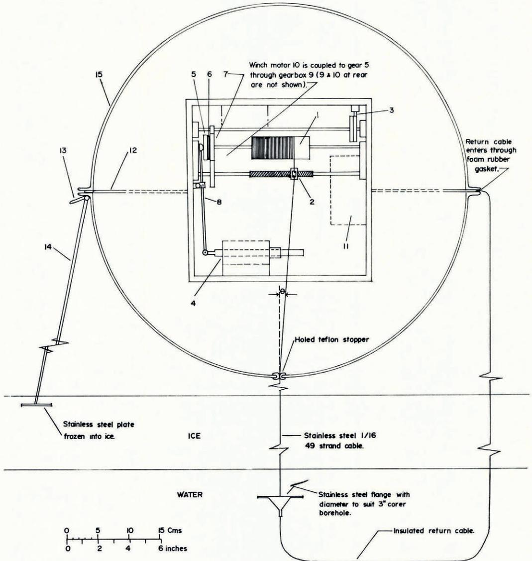
Fig. 1. Cross-section through sea-ice thickness gauge showing principles of construction and installation.
