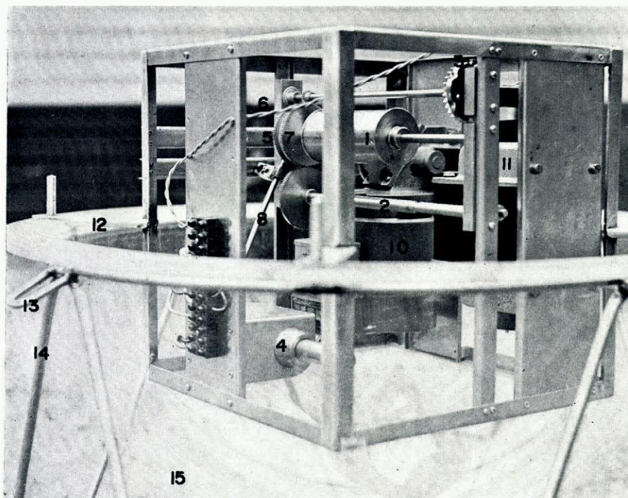
Fig. 2. Photograph of sea-ice thickness gauge with the upper perspex hemisphere and the cable removed. The key to the numbers is as for Figure 1
