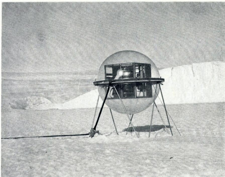
Fig. 3. Sea-ice thickness gauge installed at Mawson, showing heating light globe, power and command cable to control and recording unit on shore, with ice cliffs in the background
