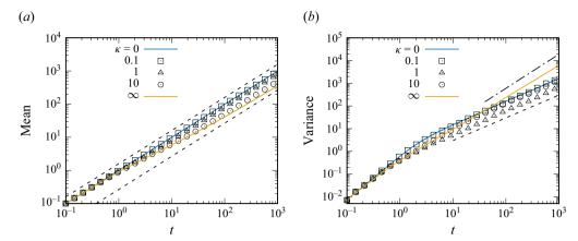
Figure 3. Displacement (a) mean and (b) variance obtained from the numerical solution of (3.26) in Gamma-distributed multi-Gaussian flow fields for  $\alpha = 3/2$  with blue solid line for  $\kappa = 0$ , squares for  $\kappa = 0.1$ , triangles for  $\kappa = 1$ , circles for  $\kappa = 10$ , and orange solid line for  $\kappa = \infty$ . The dashed lines indicate linear scaling with time, the dash-dotted line the scaling  $t^{3-\alpha}$ .
