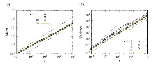
Figure 5. Displacement (a) mean and (b) variance, with triangles for  $\kappa = 0.1$ , squares for  $\kappa = 1$ , circles for  $\kappa = 10$ , and orange lines for  $\kappa = \infty$ . The dotted lines denote the expected ballistic behaviour at early times. The dashed lines indicate linear scaling with time, the dash-dotted line the scaling  $t^{3-\alpha}$ .
