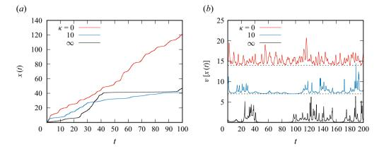
Figure 1. (a) Trajectories and (b) Lagrangian-in-time speed series for particle motion in multi-Gaussian flow fields with  $\kappa = \infty$  ( $\tau_c = 1$ , black),  $\kappa = 0$  ( $\ell_c = 1$ , red), and  $\kappa = 10$  (blue). Times and lengths are given in arbitrary units. One can clearly see the intermittent character of particle motion for the spatially varying flow ( $\kappa = \infty$ ), and the spatio-temporally varying flow below the correlation time.
