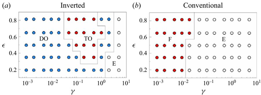
Figure 6. Mode diagram for (a) inverted and (b) conventional initial states depending on  $\gamma$  and  $\epsilon$ ; regions DO, TO, F and E correspond to the DO mode, the TO mode, the F mode and the E mode, respectively.
