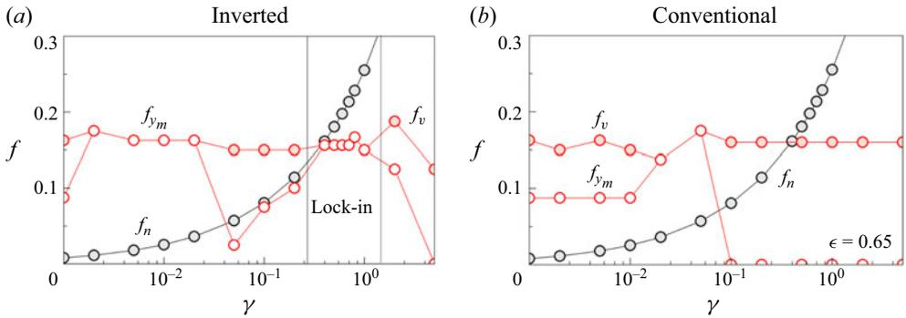
Figure 12. Oscillation frequency ( $f_{ym}$ ), vortex shedding frequency ( $f_v$ ) and natural frequency ( $f_n$ ) for (a) inverted rings and (b) conventional rings as a function of  $\gamma$  ( $\epsilon = 0.65$ ).
