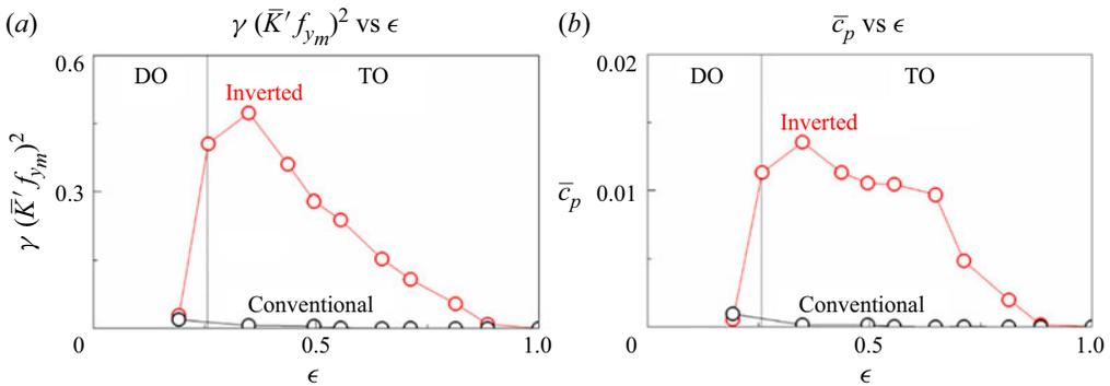
Figure 23. (a) Values of  $\gamma (\bar{K}' f_{y_m})^2$  and (b) average power coefficient ( $\bar{c}_p$ ) for inverted and conventional rings as a function of  $\epsilon$  ( $\gamma = 0.5$  for inverted and  $\gamma = 0.01$  for conventional).
