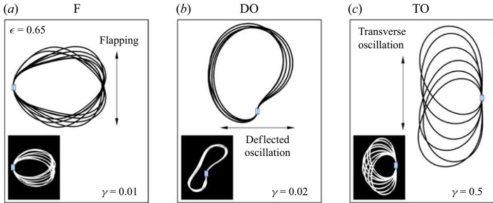
Figure 5. Superposition of the instantaneous shapes of the flexible ring for different oscillation modes: (a) F mode at  $\gamma = 0.01$ , (b) DO mode at  $\gamma = 0.02$  and (c) TO mode at  $\gamma = 0.5$ , with  $\epsilon = 0.65$ . The white line in each inset represents the experimentally observed mode.
