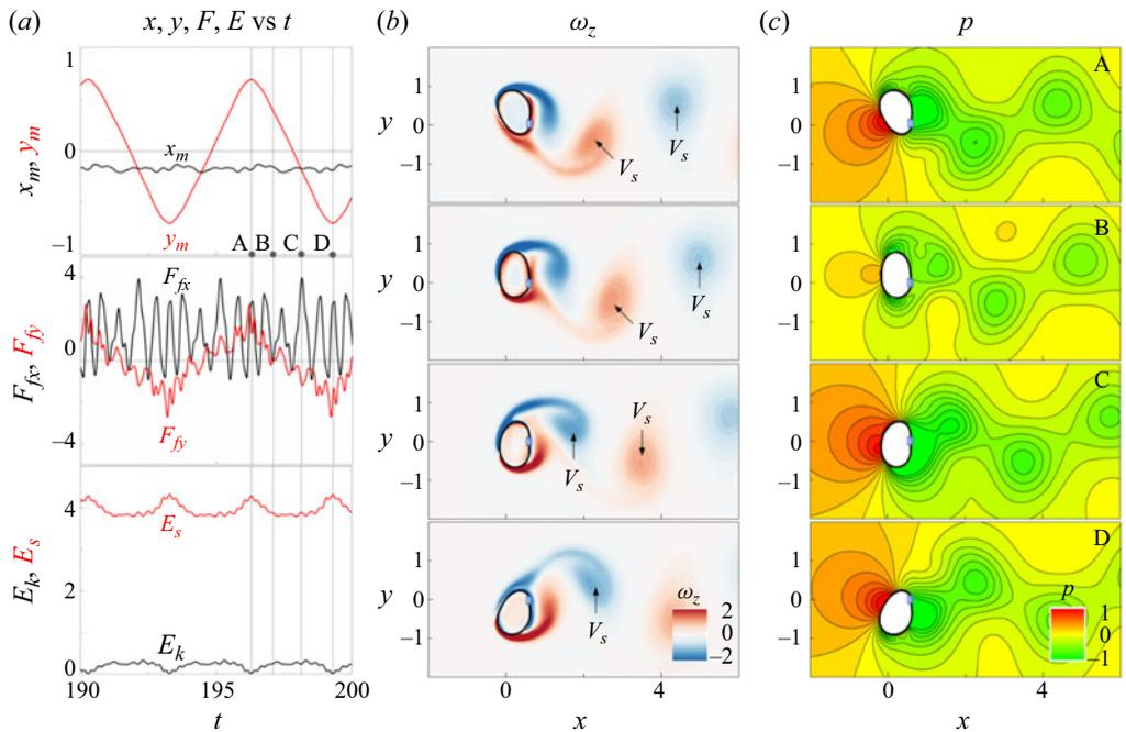
Figure 9. (a) Time histories of  $x_m$ ,  $y_m$ ,  $F$  and  $E$ . Instantaneous contours of (b)  $\omega_z$  and (c)  $p$  at A, B, C and D for  $\epsilon = 0.65$  and  $\gamma = 0.5$  under the TO mode.
