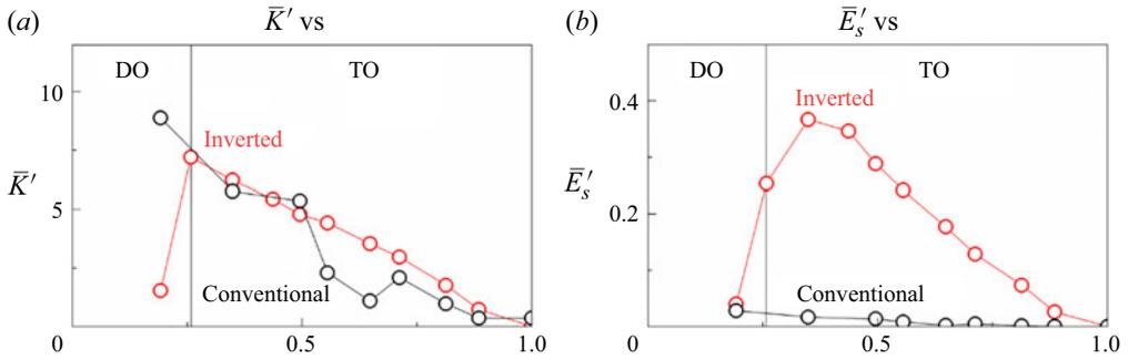
Figure 21. (a) Average variation of curvature ( $\bar{K}'$ ) and (b) elastic energy ( $\bar{E}'_s$ ) for inverted and conventional rings as a function of  $\epsilon$  ( $\gamma = 0.5$  for inverted and  $\gamma = 0.01$  for conventional).
