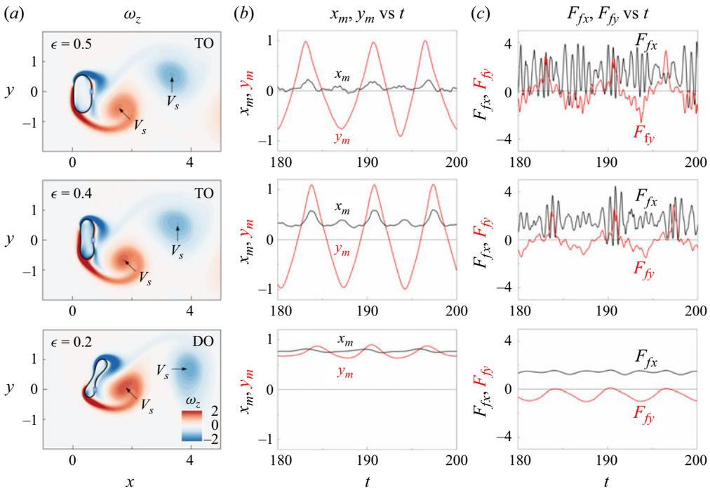
Figure 20. (a) Instantaneous contours of  $\omega_z$  and time histories of (b) the midpoint displacement and (c) fluid force for an inverted ring under  $\epsilon = 0.5, 0.4, 0.2$  ( $\gamma = 0.5$ ).
