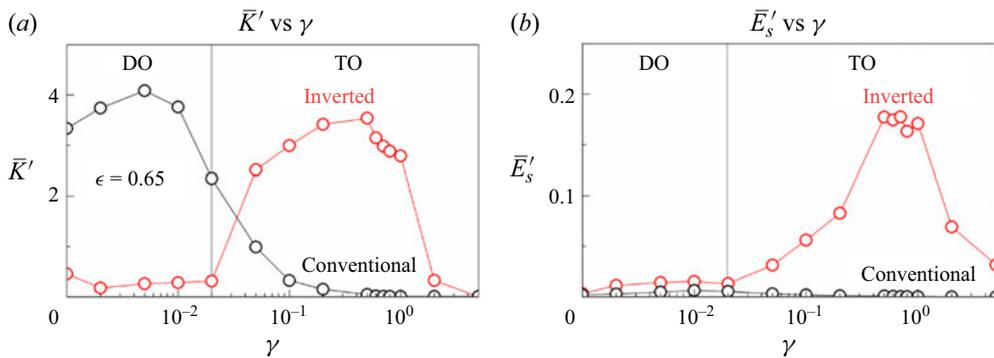
Figure 14. Average variation of (a) curvature ( $\bar{K}'$ ) and (b) elastic energy ( $\bar{E}'_s$ ) for inverted and conventional rings as a function of  $\gamma$  ( $\epsilon = 0.65$ ).
