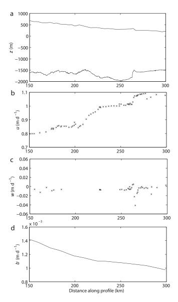
**Fig. 2.** Rutford Ice Stream data. (a) Surface and bedrock topography measured from airborne radar, (b) horizontal surface velocity, (c) vertical surface velocity and (d) water equivalent accumulation rate along the profile shown in Figure 1. The grounding line is located at the end of the profile at  $x \approx 300$  km.
