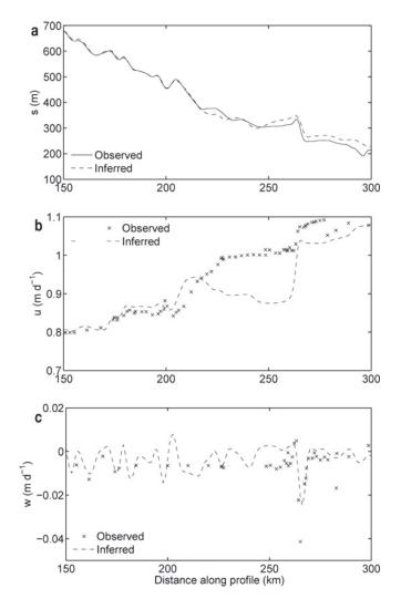
**Fig. 9.** Inversion experiment B: comparison between observed (solid curve in (a) and crosses in (b) and (c)) and inferred data (dashed curves) along the flowline on Rutford Ice Stream. (a) Surface topography, (b) horizontal and (c) vertical velocity. The inferred data correspond to the FE prediction for the MAP solution shown in Figure 7.
