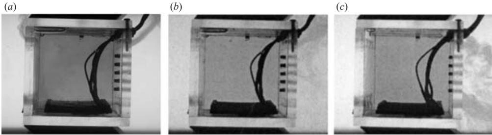
FIGURE 10. Experimentally observed regimes, for a building with three openings ( $\alpha = 1$ ). (a) The buoyancy-driven regime, with outflow from both upper vents; (b) the intermediate regime, with outflow from the upper downwind vent, and (c) the wind-driven regime, with outflow through both downwind vents.
