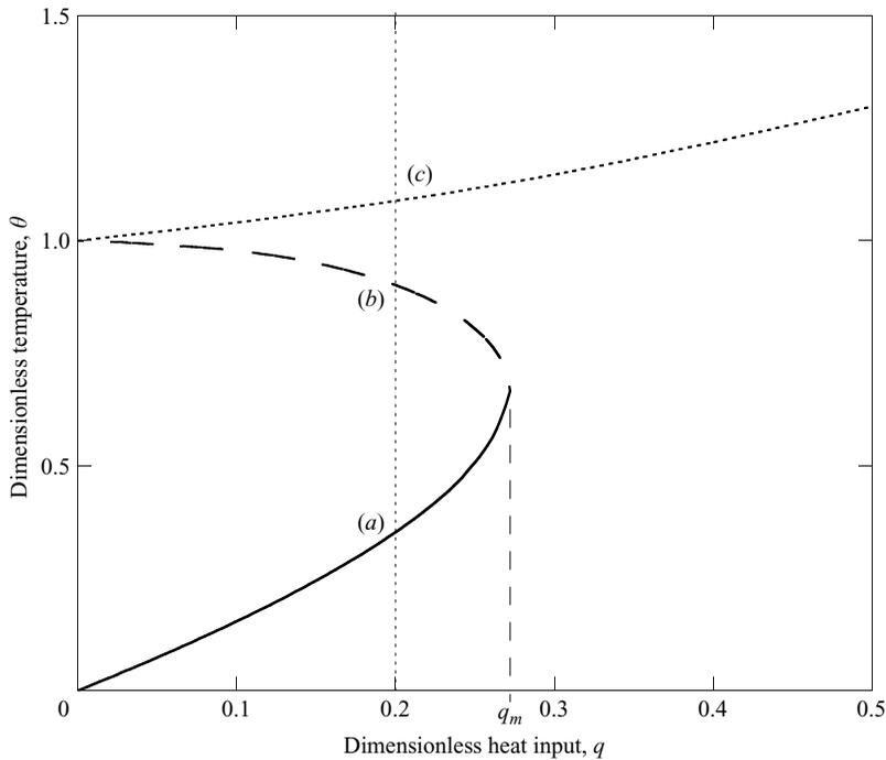
FIGURE 5. Temperature as a function of heat input for area ratio  $\alpha=0$ . The dotted line represents the buoyancy-driven regime while the dashed and solid lines represent the wind-driven regime (see figure 1).  $q_m$  is the maximum temperature at which multiple steady states are possible. The thin dotted line represents a typical heat load for which three steady states can occur; these three states are labelled (a), (b) and (c).
