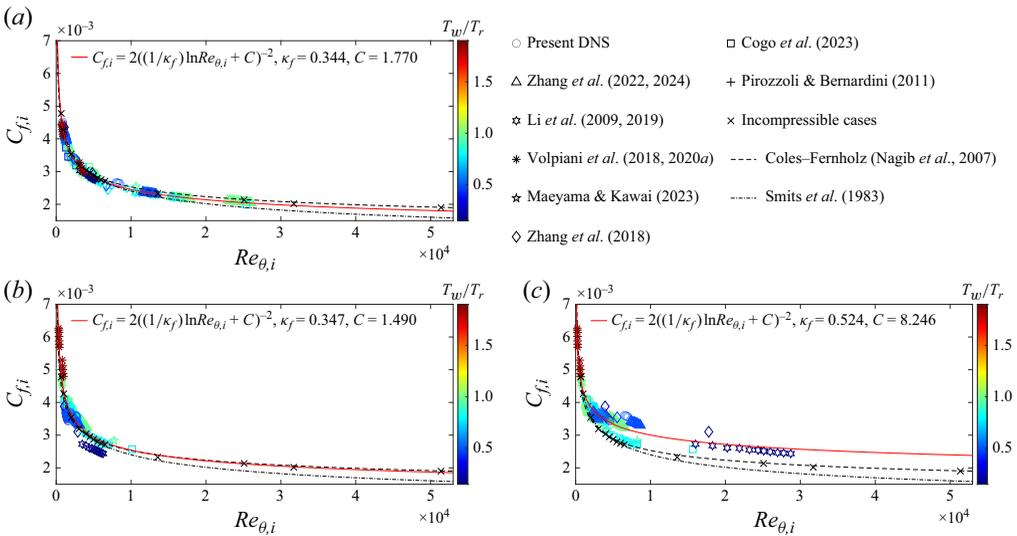
Figure 3. The transformed  $C_{f,i}$  versus transformed  $Re_{\theta,i}$ : (a) present theory, (b) vD-II theory, and (c) SC theory.
