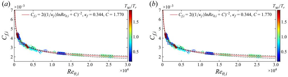
Figure 4. The transformed  $C_{f,i}$  versus transformed  $Re_{\theta,i}$  using  $\bar{U}_I$  based on (a) constant-stress-layer GFM transformation and (b) total-stress-based GFM transformation.
