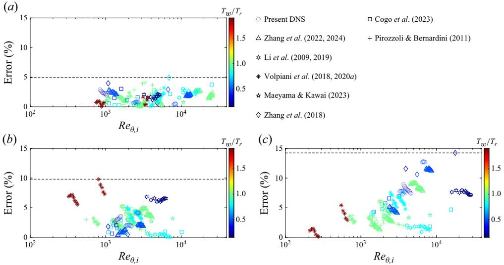
Figure 2. The error of the skin-friction coefficient, defined as  $|(2/C_{f,i})_{DNS}^{1/2} - (2/C_{f,i})_{CF}^{1/2}| / (2/C_{f,i})_{CF}^{1/2}$ : (a) present theory, (b) vD-II theory, and (c) SC theory. The black dashed line in each plot represents the maximum error.
