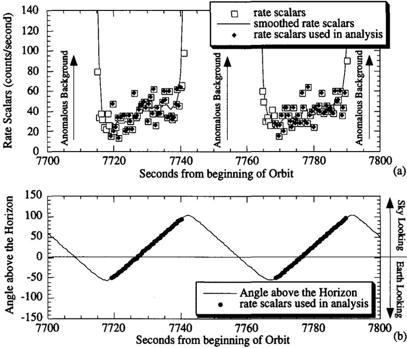
FIGURE 2. The count rate scalars (a) and the horizon angle (b) for two rotations of telescope 1B. Times dominated by the anomalous background (a) and our selected data intervals (b) are shown.
