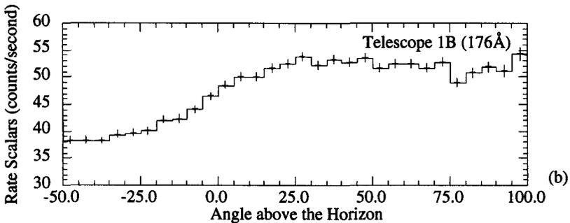
FIGURE 3. Count rates for telescope 1B as a function of the angle between the telescope's optical axis and the earth's horizon, in  $5^\circ$  bins.
