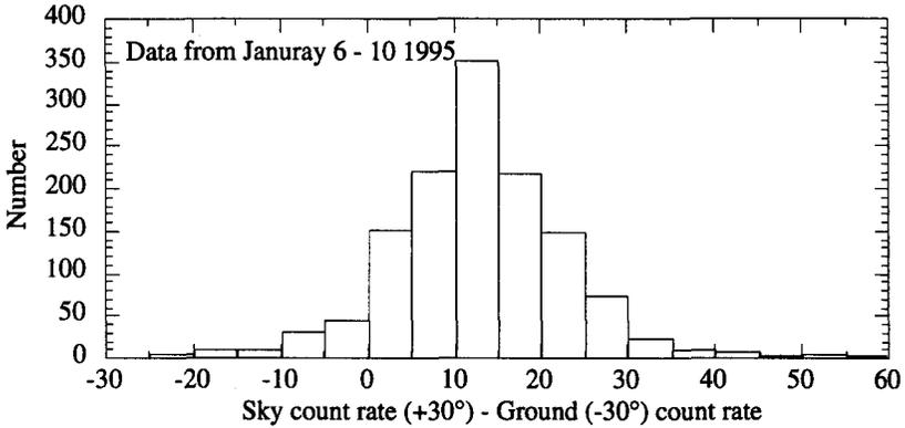
FIGURE 4. Histogram of the count rate differences between 30° above and 30° below the horizon for a data set in January.
