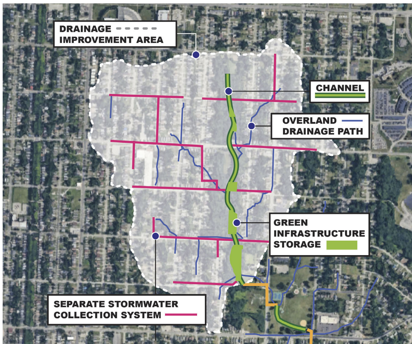
Figure 5. 37th & Norton Green Infrastructure schematic.
