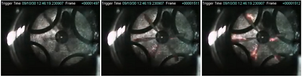
Figure 1. Single cylinder optical engine transient fuel injection consisting, from left to right in chronological order, of a starting jet, a steady-state jet and a stopping jet, during which the ignition event happens (Gill et al. 2005).
