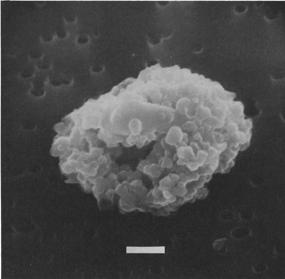
Figure 8 Chondritic micrometeorite U2-5B (24). This particle contains a moderate amount of filling material and the structure is rather typical of the chondritic micrometeorites. Scale bar = 1 $\mu$ m.
