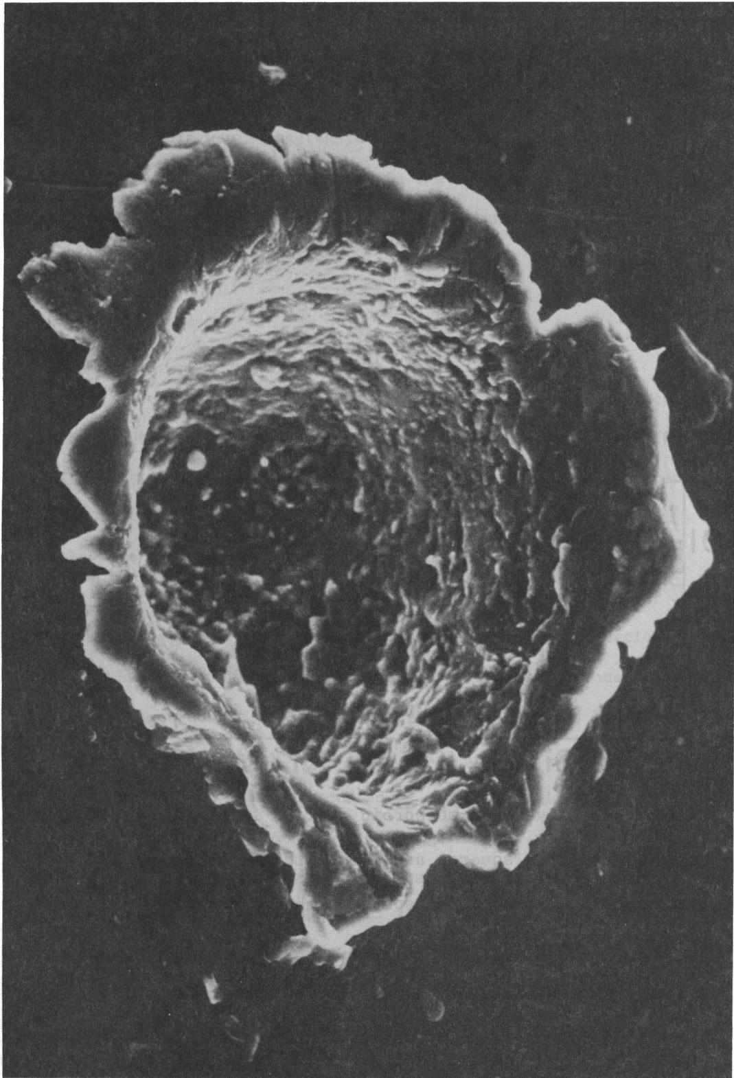
**Figure 1** 110µm diameter microcrater from Skylab IV.
