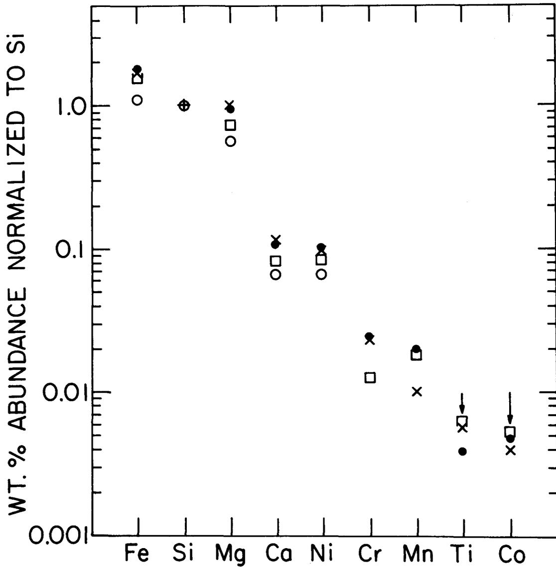
Figure 2 Microprobe analysis of meteoroid residue in the 110µm Skylab IV crater. The open squares and open circles represent independent microprobe analyses of 30µ spots on the crater floor. Filled circles and crosses, respectively, are C1 and C3 meteorite averages (Mason, 1971). Sulfur was analyzed in a separate probe run and was found to be qualitatively similar to the Fe, Mg, Si group.
