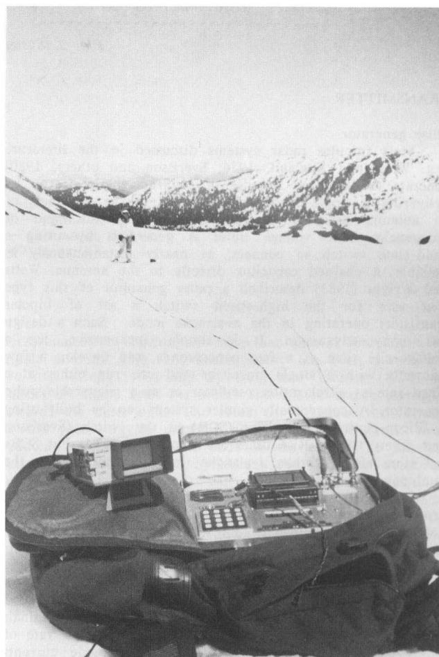
Fig. 1. Operating the U.B.C. impulse radar system from a back pack on Helm Glacier, British Columbia, Canada. Receiving unit and oscilloscope in the foreground are connected to the transmitter in the background by a fiber-optics cable.
